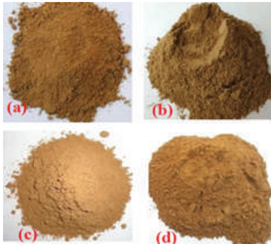
Fig. 1 Photographs of CS powder of sizes (a) 500 μm, (b) 400 μm, (c) 300 μm, and (d) 200 μm
