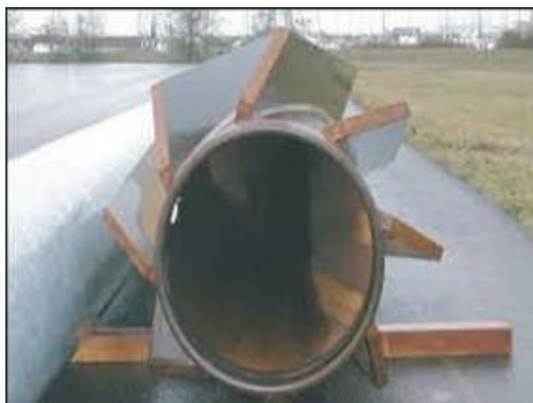
Fig. 2: Cross-section view of spin fin pie
