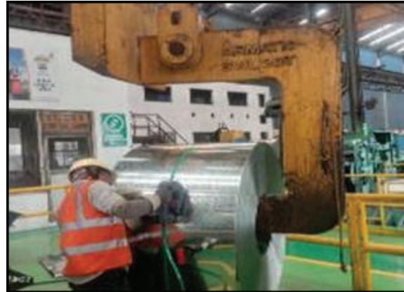
Fig. 2 (a) BOF Operation was monitored through a transparent glass window panel (b) PET strapping of coil ( Source: Tatasteel, Kalinganagar)
